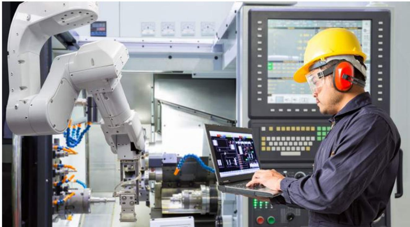
Cobots, or collaborative robots, are designed to share a workspace and tasks with humans. Instead of replacing humans, cobots augment and enhance human capabilities with strength, precision, and data capabilities. Cobots are trained differently than traditional industrial robots. Rather than programmed to a specific set of steps using programming tools, many cobots are trained by humans manipulating the arms and training by example.
